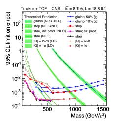
► CMS/ATLAS can search for stable massive long-lived particles with time of flight analysis and search for anomalous energy loss in tracker figure from CMS [1305.0491]
