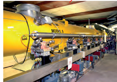
Accelerator modules 150 – 450 – 1250 MeV
