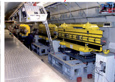
Undulator Assembly NdFeB, Length 6 x 4.5 m Magnetic period 27 mm Fixed Gap 12 mm
