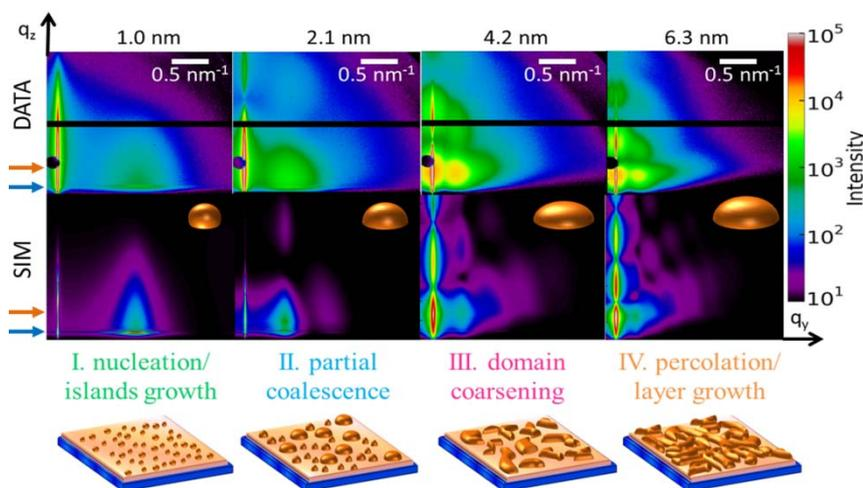
Figure 1: Sputter deposition of Au on PS. **Upper row:** Selected 2D GISAXS patterns with increasing effective Au film thicknesses  $\delta_{Au}$ . The critical angles of PS (blue) and Au (orange) are indicated by arrows. **Middle row:** model-based simulation of the GISAXS pattern, based on the object shape sketched in the upper right corners. **Lower row:** Sketch of the cluster growth morphology with ongoing sputter deposition in the four stages of growth. See [4].
