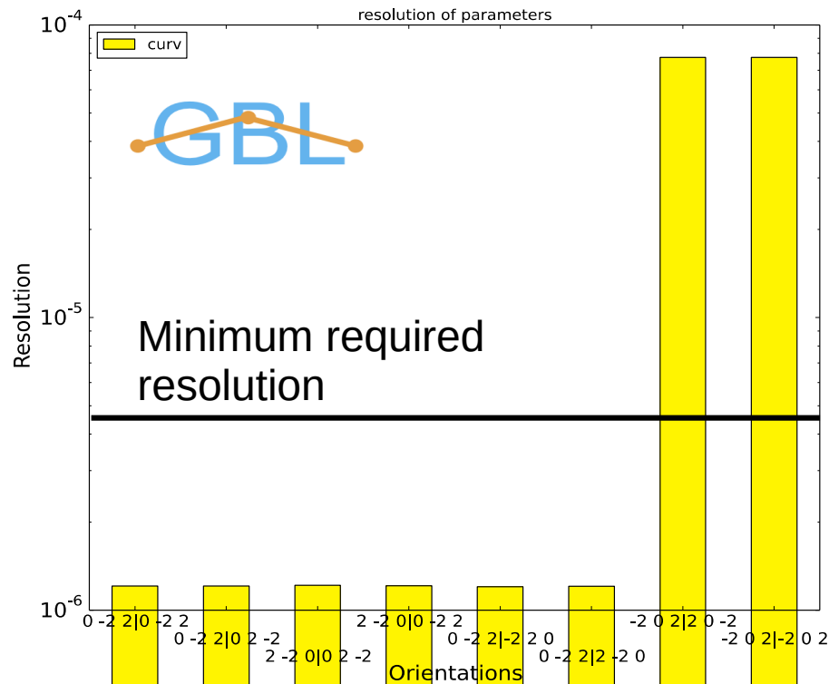
Fig.: Achievable curvature and z resolution of the telescope, with multiple scattering, depending on angular orientation
