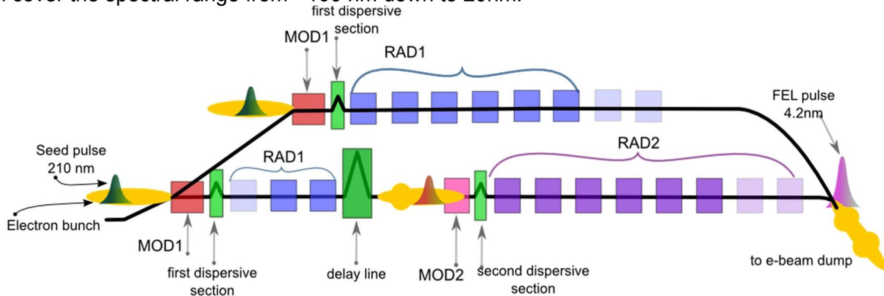
FEL-2, in order to be able to reach the wavelength range from 20 to  $\sim 4$  nm starting from a seed laser in the UV, will be based on a double cascade of high gain harmonic generation. The nominal layout will use a magnetic electron delay line in order to improve the FEL performance by using the fresh bunch technique. Other FEL configurations are also possible.
