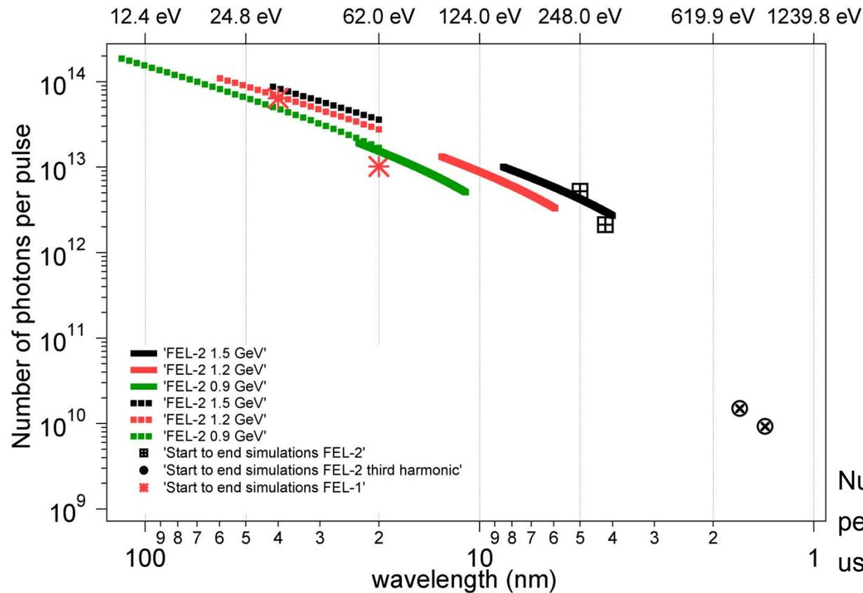
Numerical predictions of the FEL performance based on M. Xie formulae using the FERMI parameters
