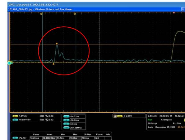
After the signal optimization using a CCD it has been possible to obtain the timing parameters that allow to overlap in time e-beam and seed laser within +50 ps
