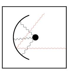
faster but less sensitive: broadband search w/o resonant enhancement: collect light at center of reflecting sphere Jaeckel/Redondo more info:[1212.2970] and [1308.1103]
