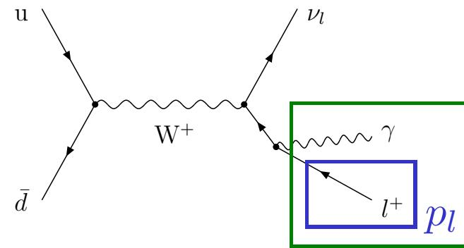
$$p_l = p_l + p_\gamma \quad (\text{for collinear photons})$$
