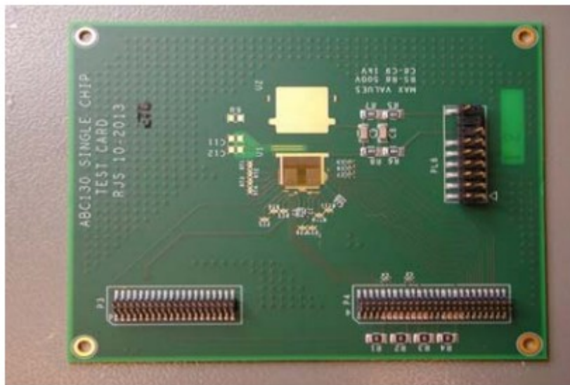
The single chip readout board and associated driver board
