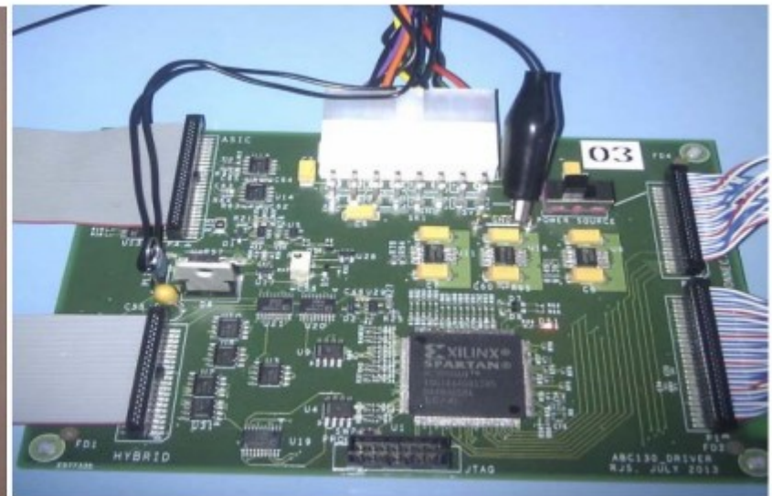
The single chip readout board and associated driver board
