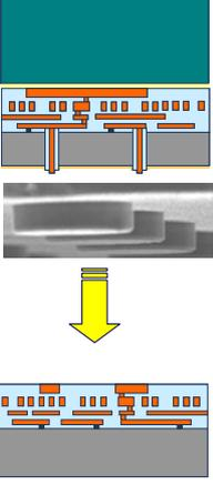
**Mixed polymer and Cu-Cu thermocompression bonding**
