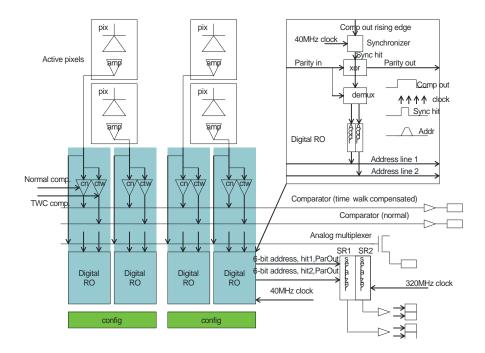
Figure 2: Detailed block scheme of the AMS H35 test chip.
