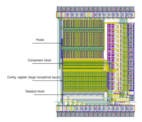
Figure 4: Layout of the AMS H35 test chip for the ATLAS strip detector.
