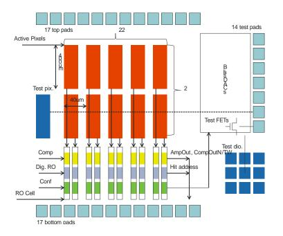
Figure 1: Block scheme of the AMS H35 test chip for the strip detector.
