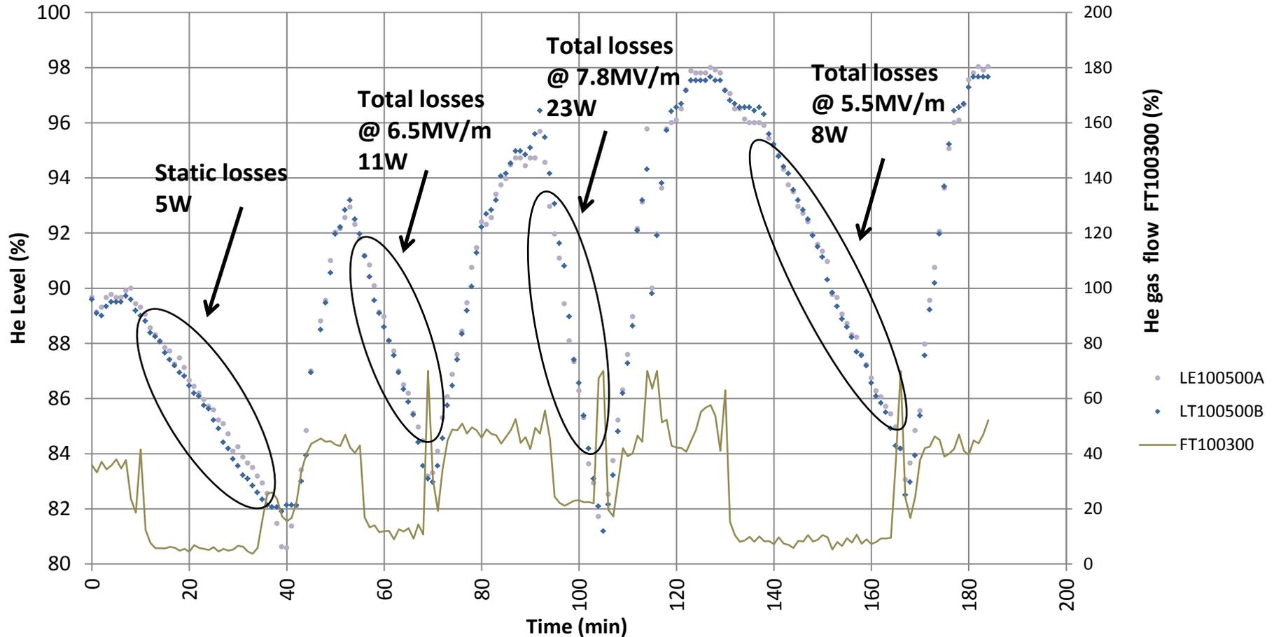
Using Lhe level gauge rate of change in the upper part of cylindrical He jacket/phase separator (Boil-off)
