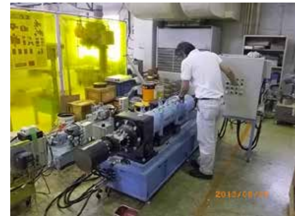
Hydroforming machine (Final hydraulic pressure: 25 MPa)
