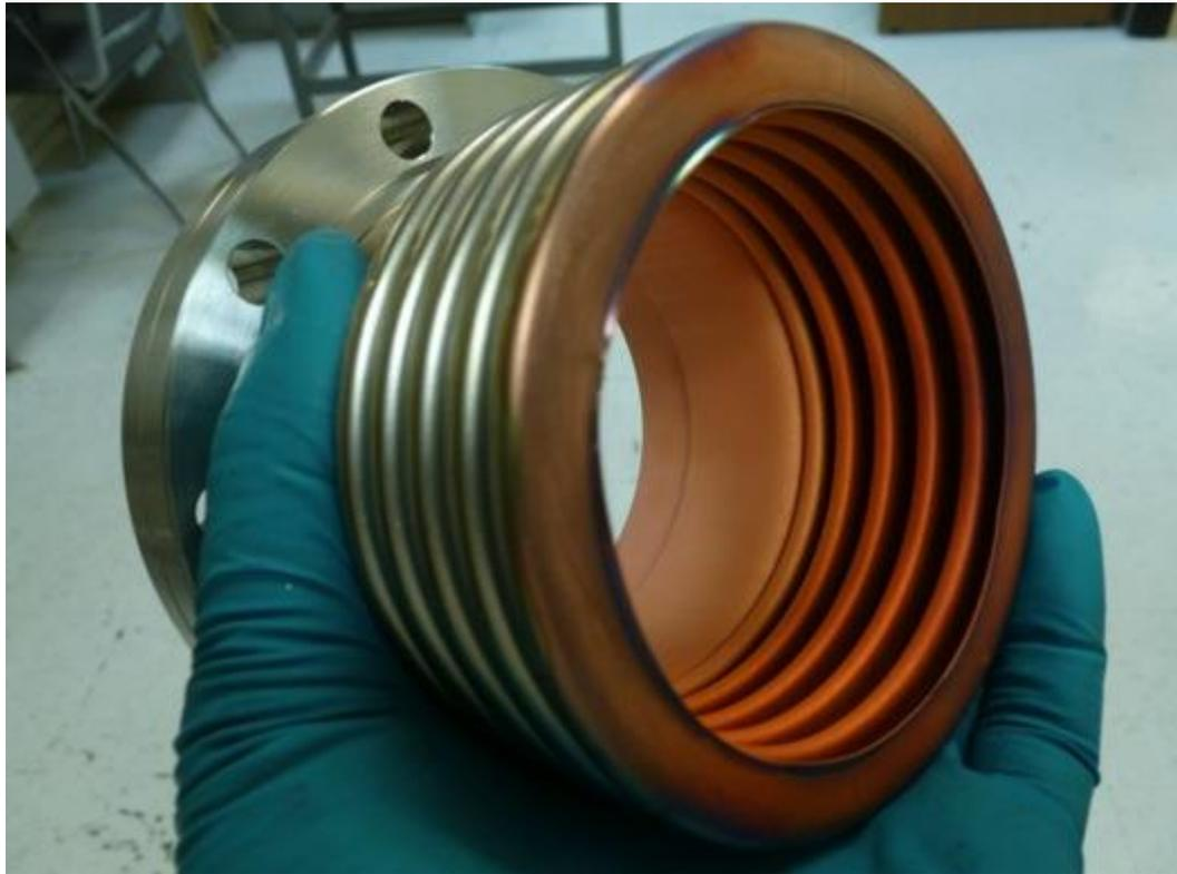
Stainless steel bellows coated with a  $\sim 45\mu\text{m}$  Cu film using the AASC CED process
