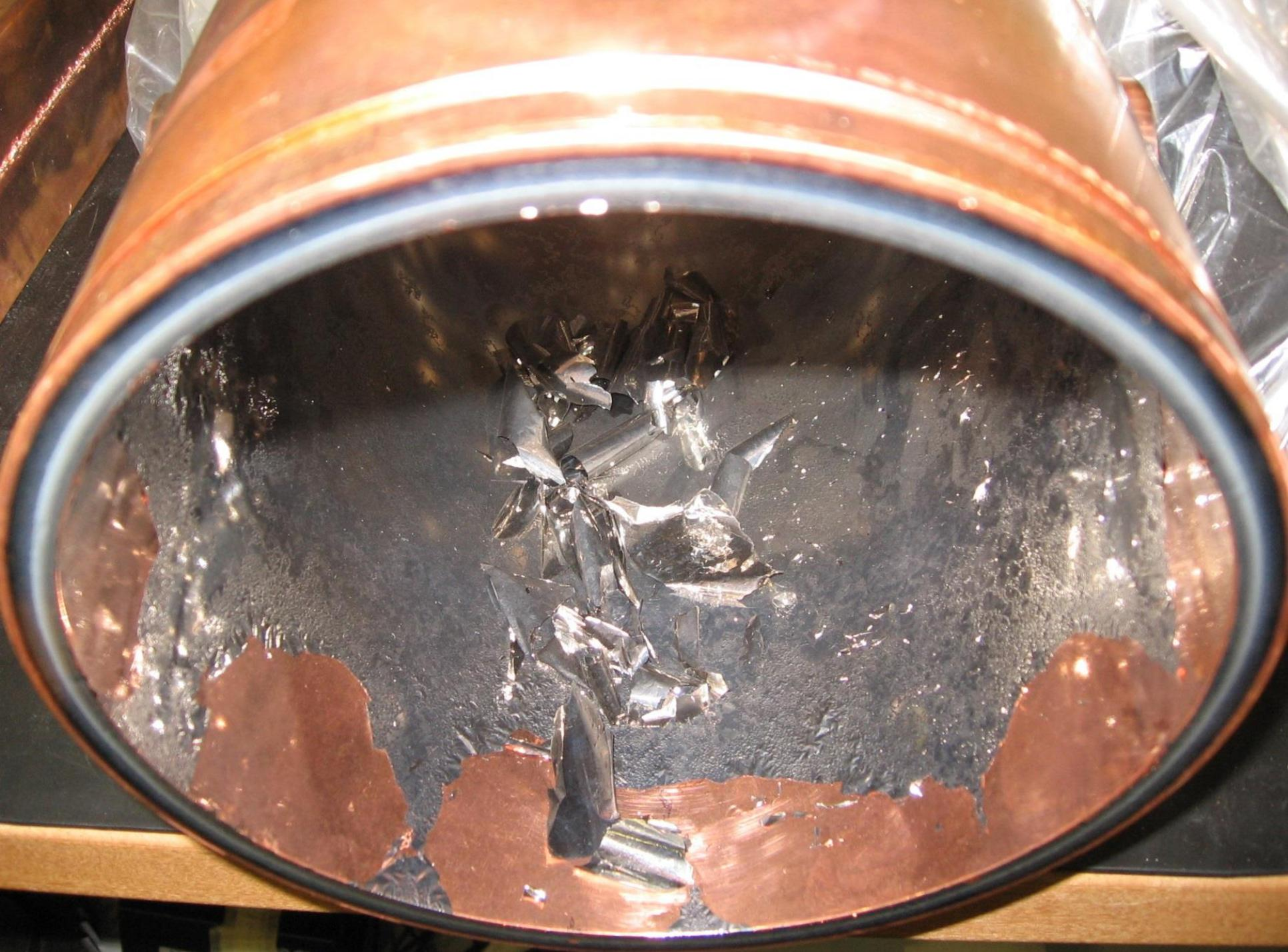
**The Cathodic Arc coated cavity deposited by Soltan Institute
