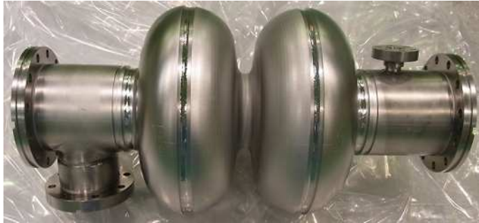
MHI-B cavity VT result at JLab
