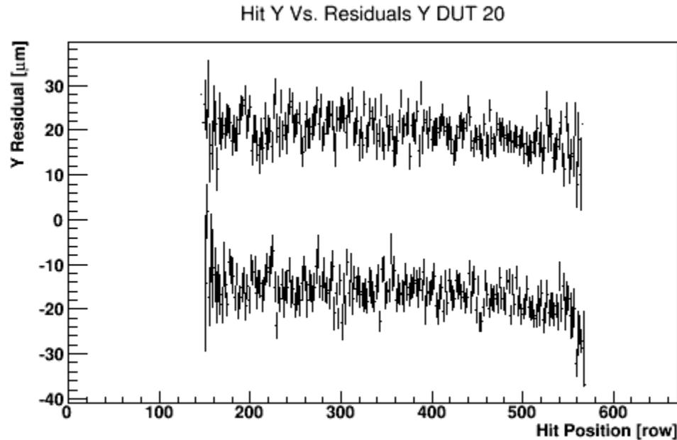
For each hit position, two residual values ( $\sim \pm 15\mu\text{m}$ ) exist...
