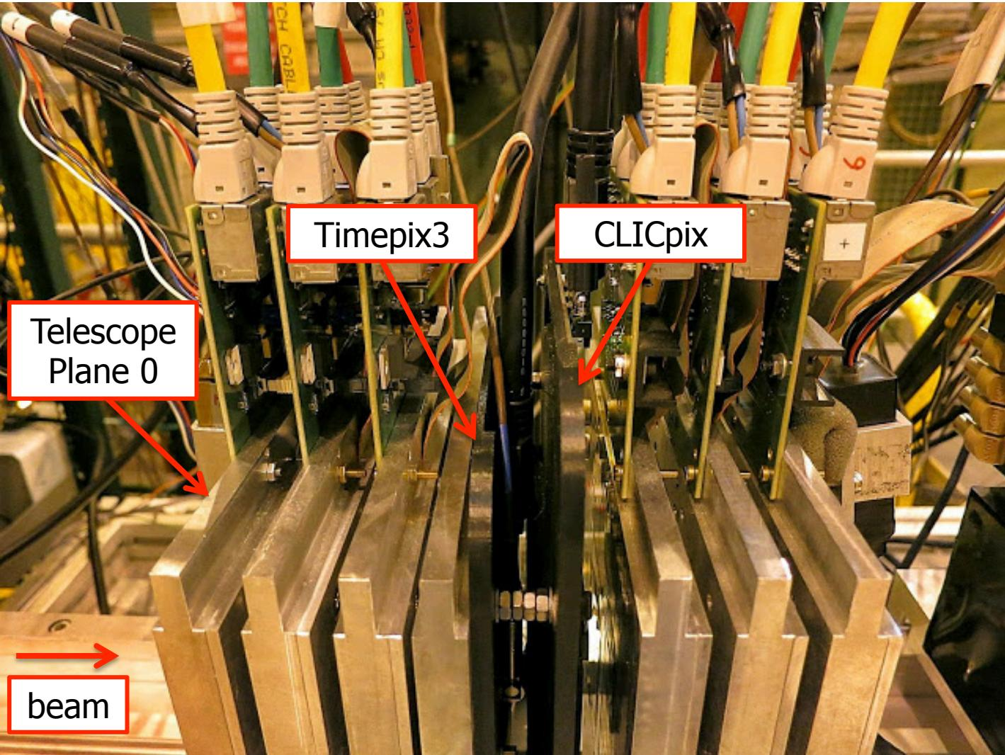
Compact telescope configuration is optimal for high momentum beam
