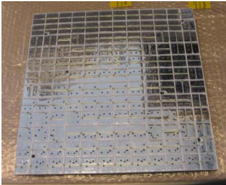
Bottom view (channels are wrapped in reflector foil)
