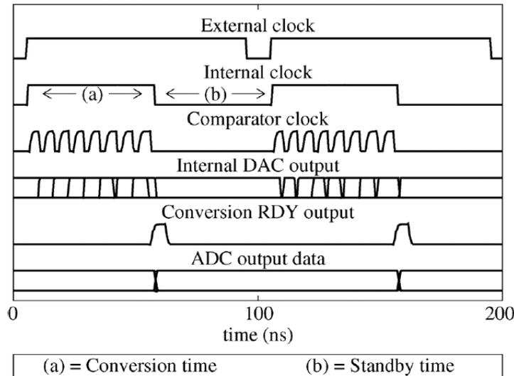
Asynchronous ADC timing
