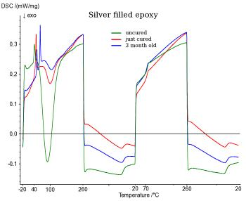
several glues measured with differential scanning calorimetry
