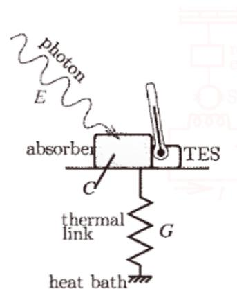
Tungsten chip (25 x 25  $\mu\text{m}$ , 20 nm)
