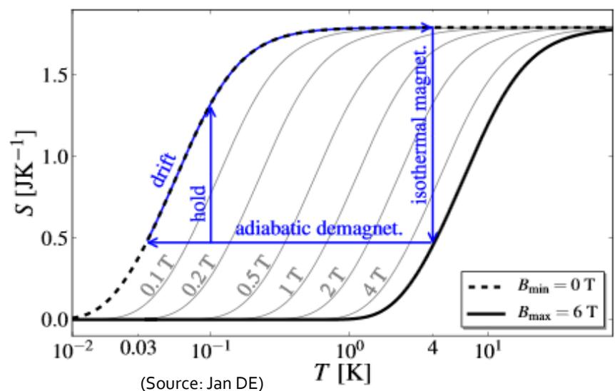
D. Wernicke , Entropy GmbH: Closed-cycle cryostats for the Kelvin and milli Kelvin temperature range
