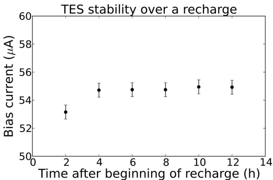
*The TES bias current equivalent to  $R_0 = 30\% R_{normal}$  as a function of time after the beginning of a recharge.*
