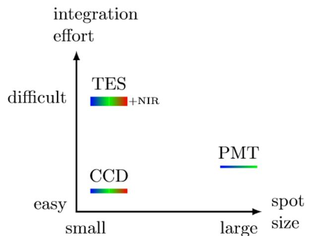
The TES and CCD weak point comes from the necessity of a good beam focusing on the chip.
