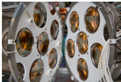
Setup to test 250 PMTs for XENON1T
