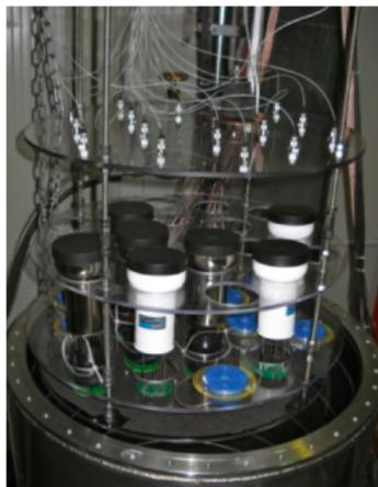
PMT tests at Naples Cryo-Lab
