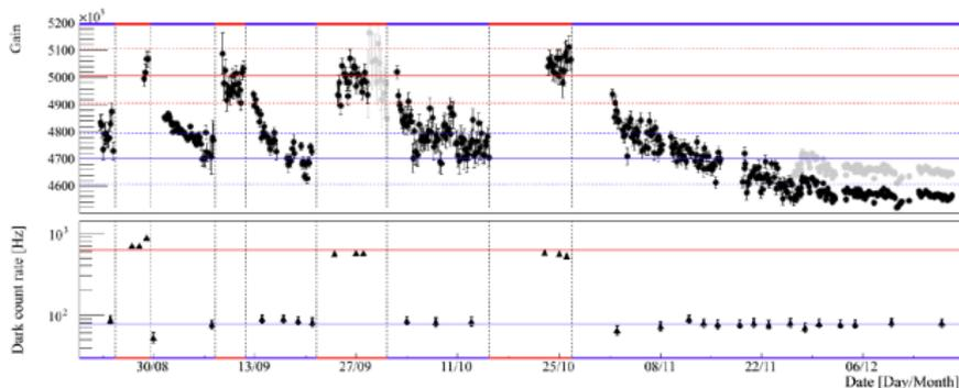
Thermal cycling of a R11410 PMT
