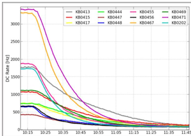
Example of PMT dark-count rates during cooling down
