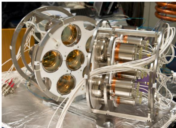
XENON1T testing setup for R11410-21 at MPIK
