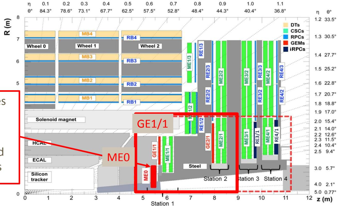
Extended coverage provides muon tag in forward region  $|\eta| < 3$
