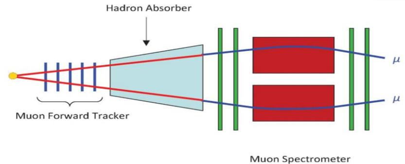
**Upgrade: Addition of a detector based on pixel CMOS sensors (MFT)** in the Muon Spectrometer acceptance to improve muon physics capabilities:
