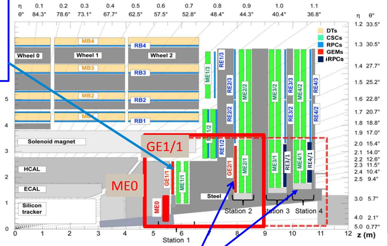
Enhance region without redundancy  $1.6 < |\eta| < 2.4$  with **maximum rate**. Technology = GEM (GE2/1) and improved high-rate RPC (RE3/1 and RE4/1)
