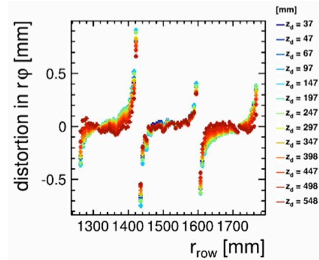
measured distortions after alignment, but with local field distortions
