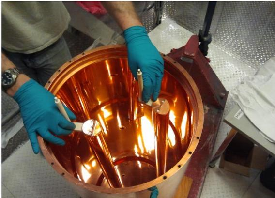
Cavity with lid off, showing tuning rods
