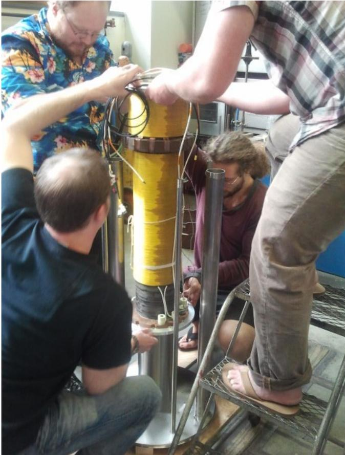
Installation of bucking coil
