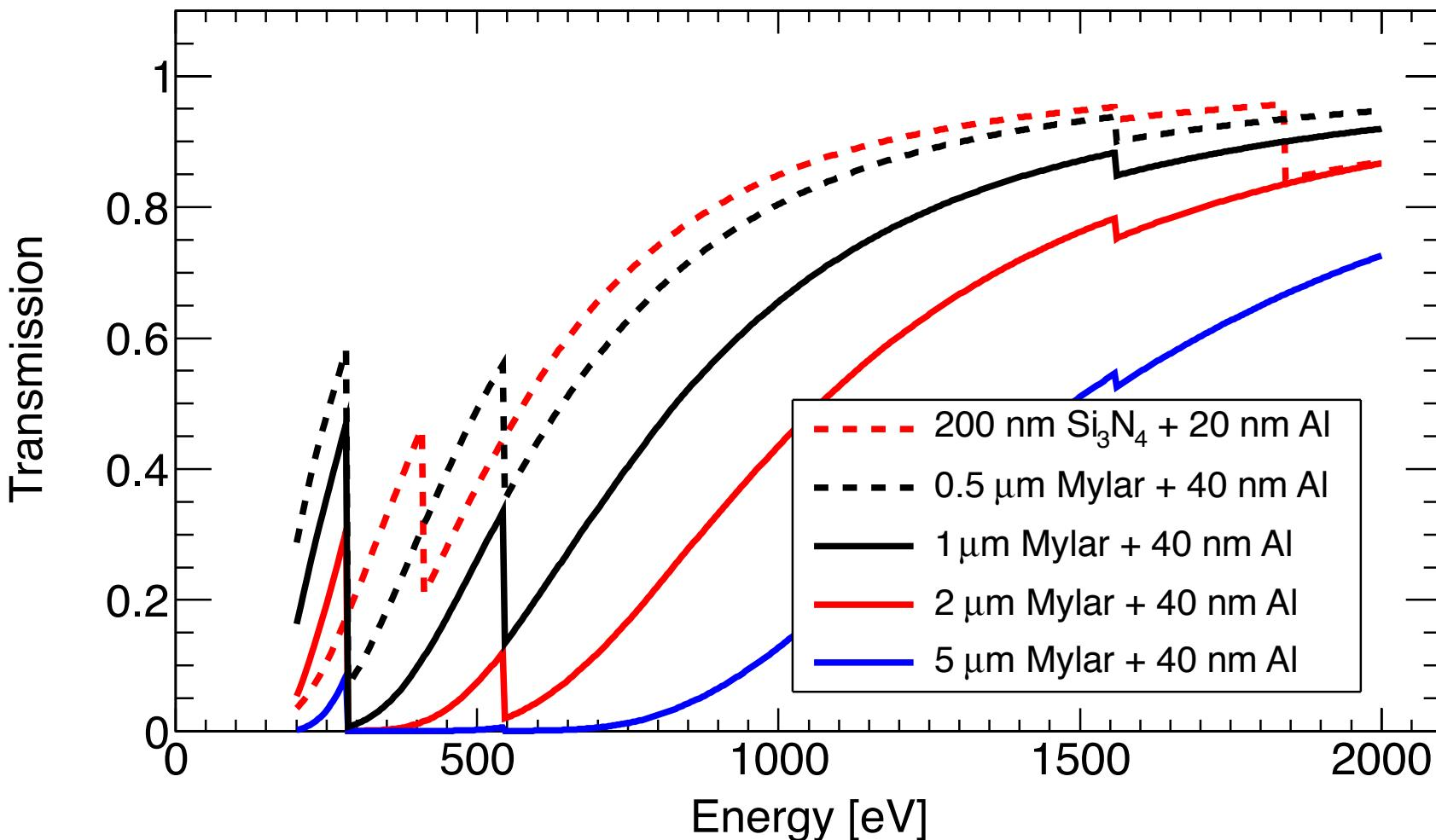
Currently: 2  $\mu\text{m}$  Mylar (aluminized) + Cu strong-back
