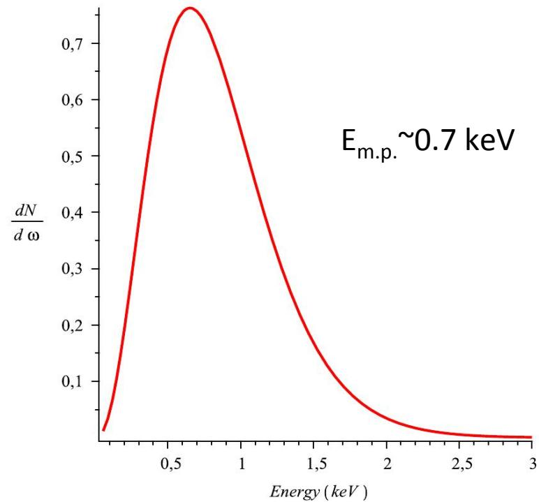
→ need X-ray detector sensitive to sub-keV photons
