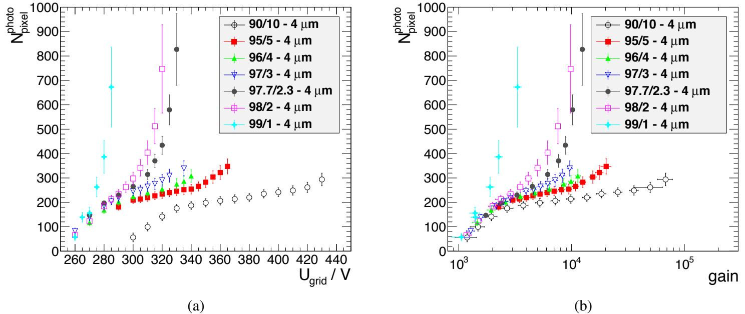
Figure 9.2: Dependence of the number of pixels over threshold in the photo peak on the grid voltage  $U_{\text{grid}}$  (a) and the gas gain (b) for different Ar/iC<sub>4</sub>H<sub>10</sub> mixtures. All error bars are inflated by a factor of 100.
