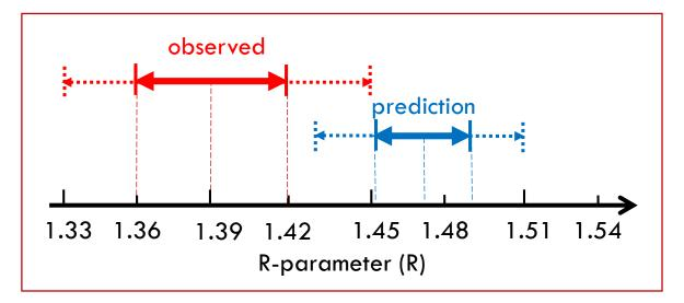
Using recent measurements of the helium mass fraction one would predict R = 1.47, a value somewhat higher than the observed  $R = 1.39 \pm 0.03$ .
