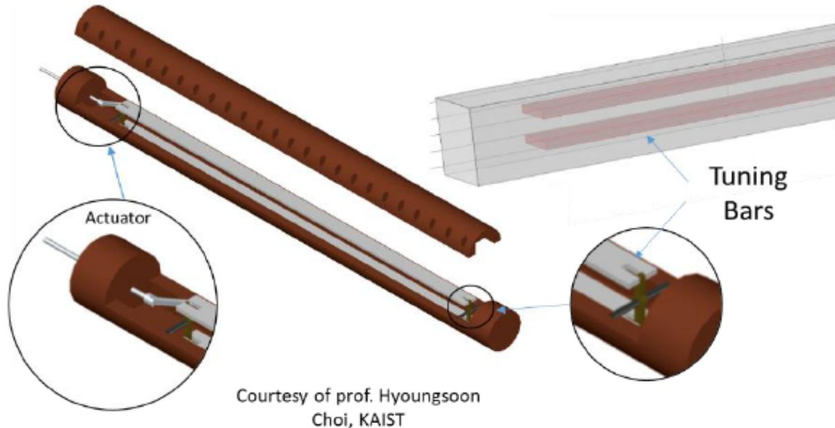
**Figure 3:** Conceptual engineering design of a possible tuning solution for a 2.5cm x 2.4cm X 50cm prototype cavity with dielectric tuning bars. The cavity is tuned by one single piezo actuator placed externally, while the bars are kept parallel to each other. This image does not necessarily represent the way in which the cavity will be assembled.
