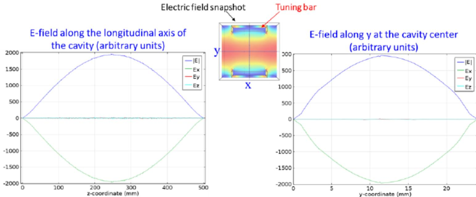
**Figure 6:** The electric field inside the resonator when the dielectric tuning bars are at a distance of 1 mm from the cavity walls. Notice how the electric field distribution is altered by the presence of the tuning bars. The field is more intense in the red, compared to the yellow, areas of the XY map (inset).
