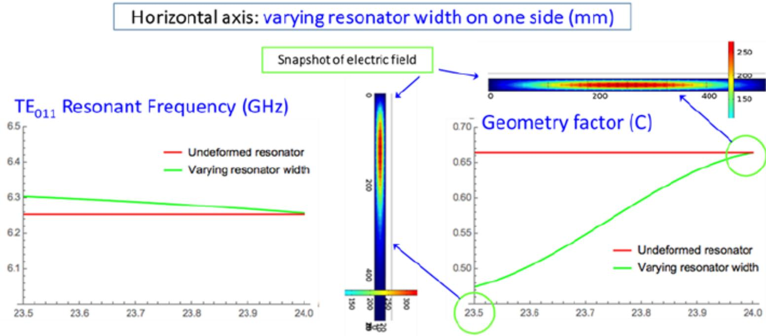
**Figure 7:** Mechanical tolerances and mode localization in a 2.5cm x 2.4cm x 50cm cavity.
