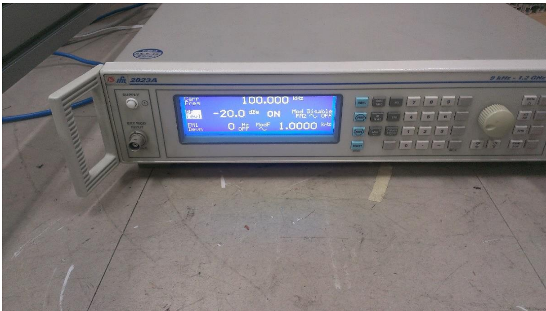
Signal generator Fluctuation of local frequency → Need for calibration
