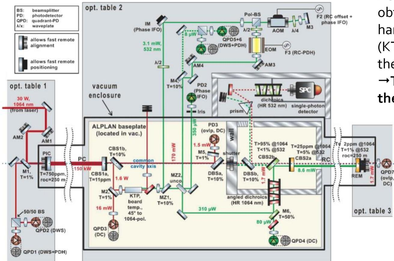
Auxiliary green beam obtained via second harmonic generation (KTP crystals) from the IR production.
