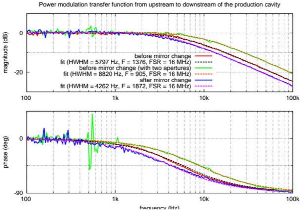
The PB of the production cavity is not sufficient ( $< 5000$ ).
