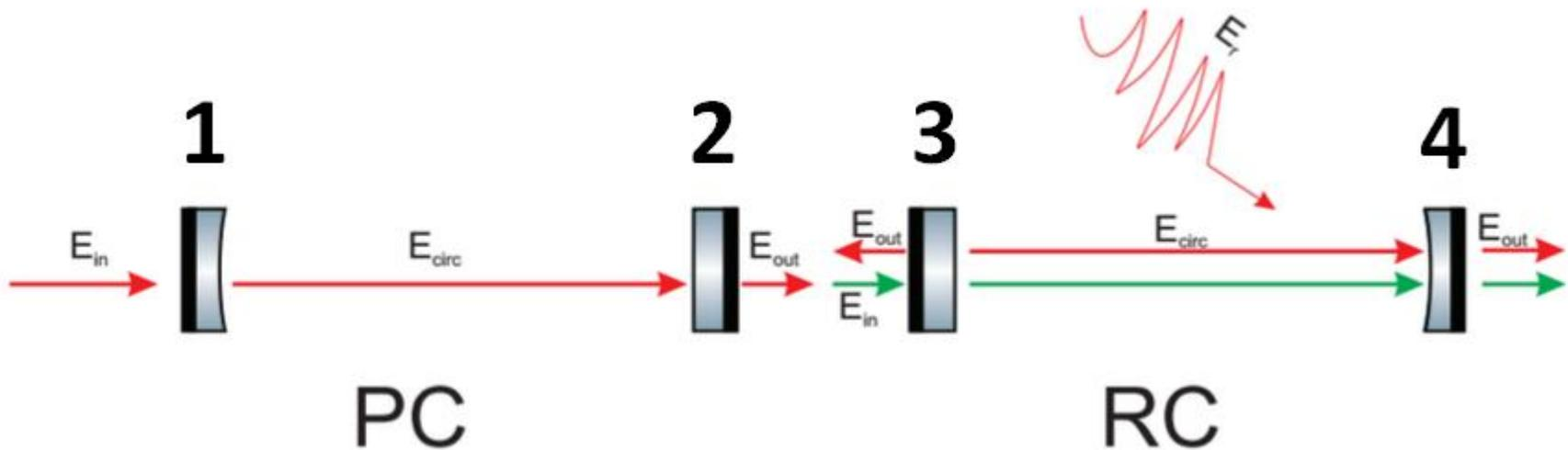
The PC and the RC needs to be in the same modal phase in order to reach the highest PB (aiming for 95% mode overlap).
