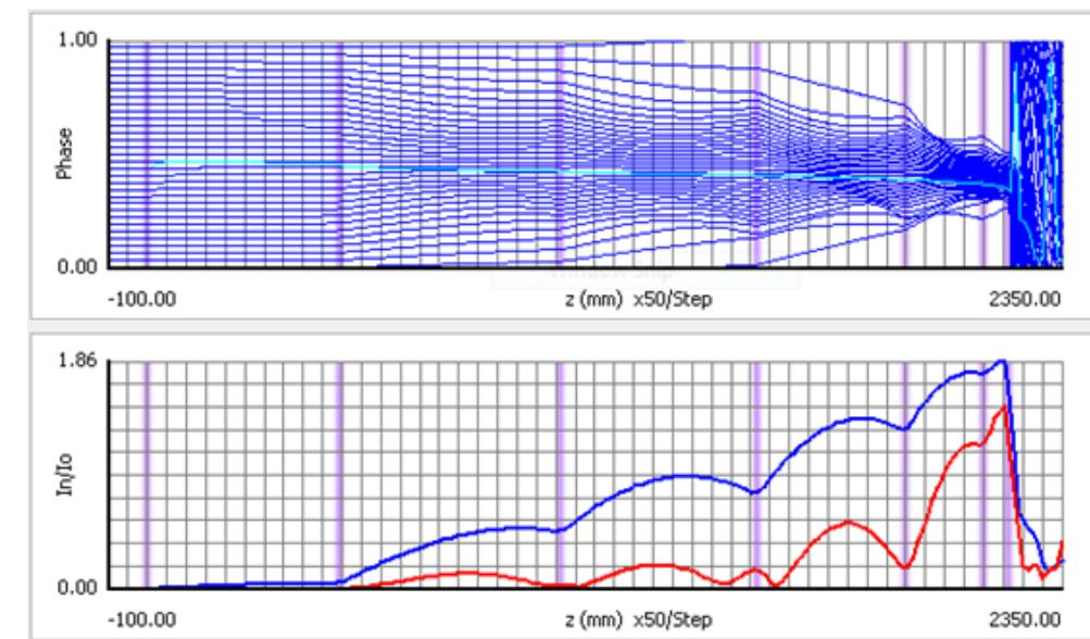
The first 'robust' (2D) design with 82% RF production efficiency. Klys2D code **THALES**
