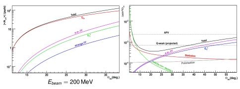
→ Optimal measurement for E = 155 MeV,  $\theta_e = 35^\circ \pm 10^\circ$  $\langle Q \rangle = 0.067$  GeV SM prediction:  $A_{LR} = -2.8 \times 10^{-8}$ , precision goal: 1.5%  $\Delta \sin^2 \theta_w = \pm 0.00031$ , i.e. 0.13 % Polarization asymmetry including higher-order corrections:
