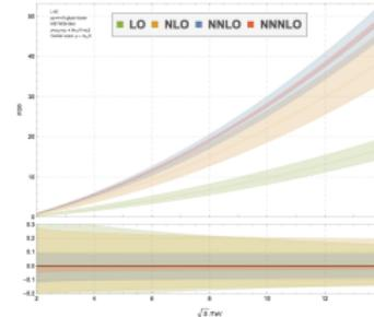
FIG. 3: The gluon fusion cross-section at all perturbative orders through N<sup>3</sup>LO in the scale interval  $[m_t^\mu, m_H]$  as a function of the center-of-mass energy  $\sqrt{s}$ .
