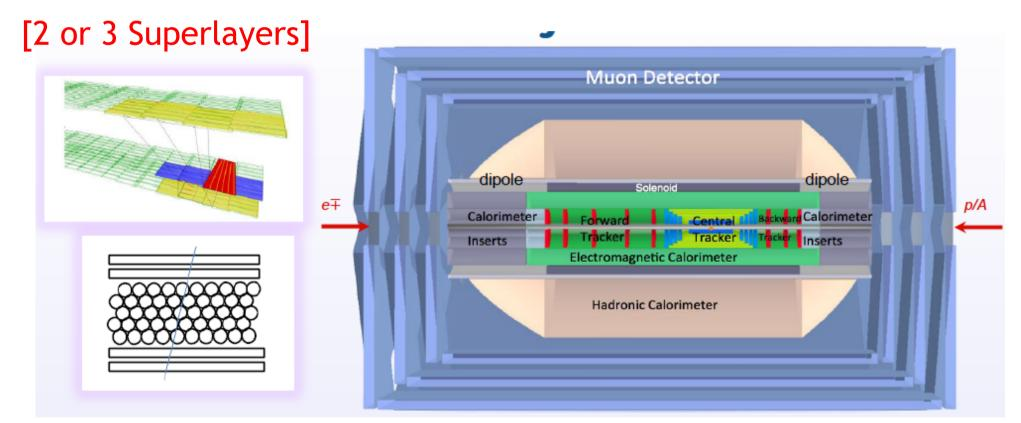
[Drift tubes / Cathode strip chambers  $\rightarrow$  precision Resistive plate / Thin Gap chambers  $\rightarrow$  trigger + 2<sup>nd</sup> coord]
