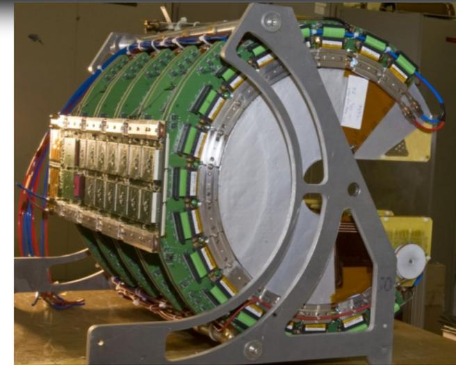
An assembled quarter of one T2 Telescope
