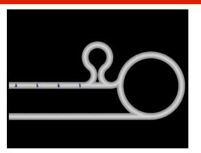
Delay loops create drive beam bunch-structure
