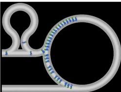
Low energy high current drive beam -> high energy low current main beam
