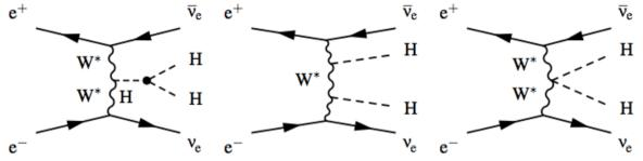
Looking at HHvv -> bbbbvv 4-jet final state, require 4 b-tag jets -> systematic studies of clustering and jet algorithm to optimize for energy flow
