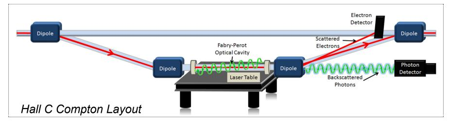
JLab has built two similar Compton polarimeters in Halls A and C  $\rightarrow$  Both have achieved ~1% electron beam polarization measurements
