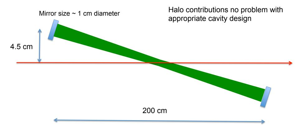
Electron-laser crossing angle = 2.58 degrees Mirror radius of curvature = 120 cm Laser size at cavity center  $(\sigma_x, \sigma_y)$  = 151.4 um
