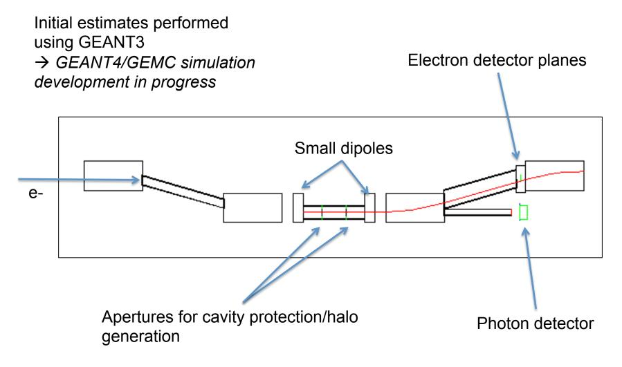
Realistic beam sizes from machine design used
