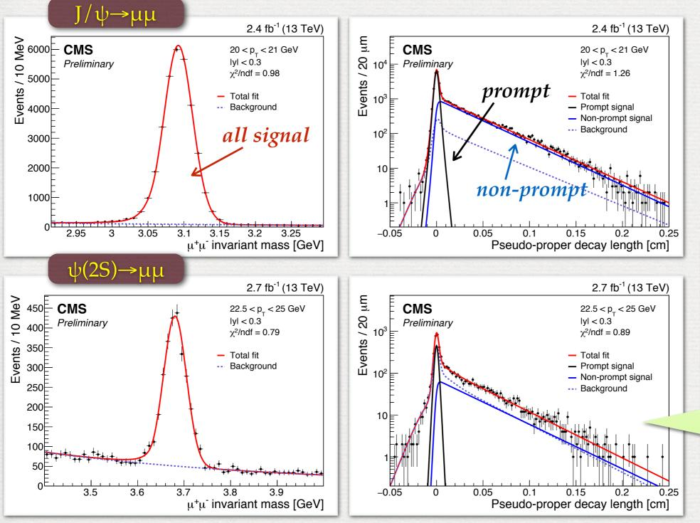
Charmonium: 2D fits to **invariant mass** and **decay length** are used to obtain the *signal yields* and *non-prompt fractions* together.
