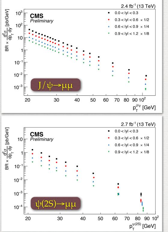
Differential cross sections measured in 4 rapidity bins. Extending up to 120 GeV in pT for  $J/\psi$ , and up to 100 GeV for  $\psi(2S)$ .
