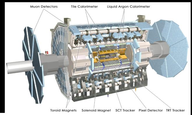
**η coverage**: Inner Tracker (-2.5, 2.5) Muon Spectrometer (-2.7, 2.7) EM Calorimeter (-3.2, 3.2) HAD Calorimeter (-4.9, 4.9)
