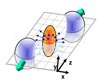
Anisotropic spatial collective motion is described by a Fourier expansion of particle distribution in azimuthal angle  $\boldsymbol{\phi}$
