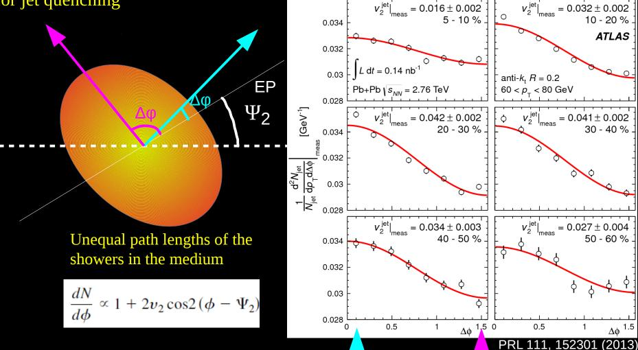
Jets produced in the direction of the event-plane are less suppressed
