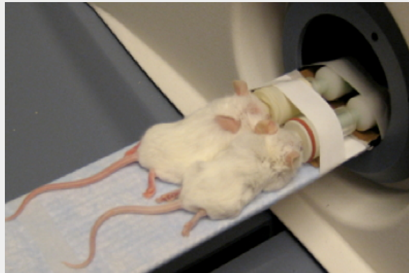
Increasing Throughput: Side-by-Side Mouse Imaging 32 g and 28 g Mice
