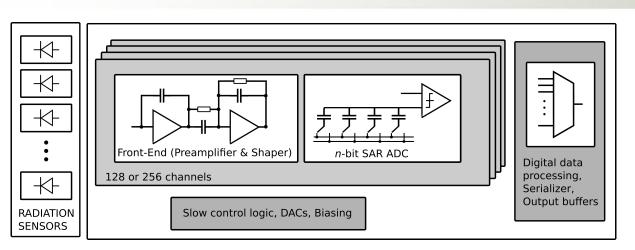
We are developing ultralow power readout ASIC with good amplitude and time measurement for LumiCal detector
