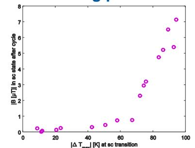
Direct measurement of the frozen thermoelectric fields in the cavity. Higher temperature differences generates higher fields..
