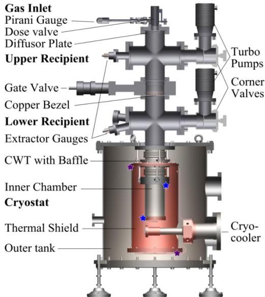
Pumping properties of cryogenic surfaces are investigated with a dedicated measurement setup
