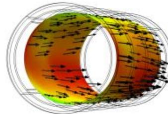
Simulation shows magnetic fields of >10 μT at the RF surface, generated by an asymmetric distributions of the thermocurrents
