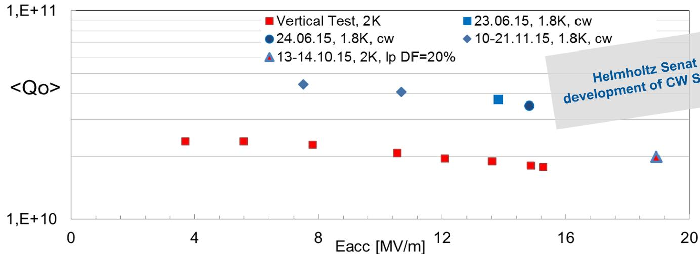
Accelerating gradient  $\langle E_{acc} \rangle$  in [MV/m] demonstrated for 3 operation modes
