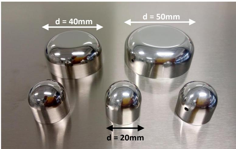
Test electrodes from polished stainless steel and aluminum
