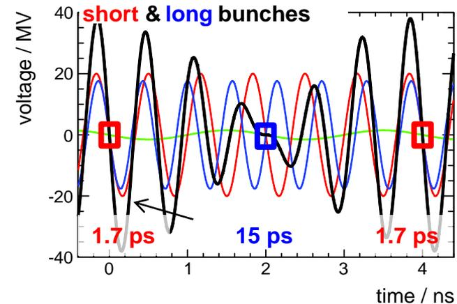
Installed voltage: 20 MV @ 1.5 GHz
