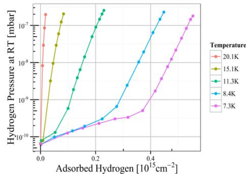
Adsorption isotherms are measured for different temperatures → included into dynamic vacuum simulations
