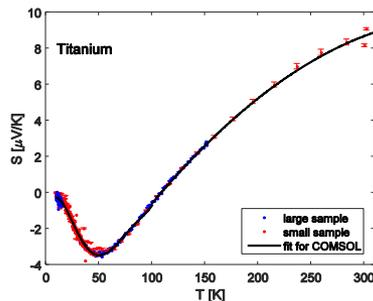
Seebeck-coefficient (measure of thermoelectric effects) determined at low temperatures.
