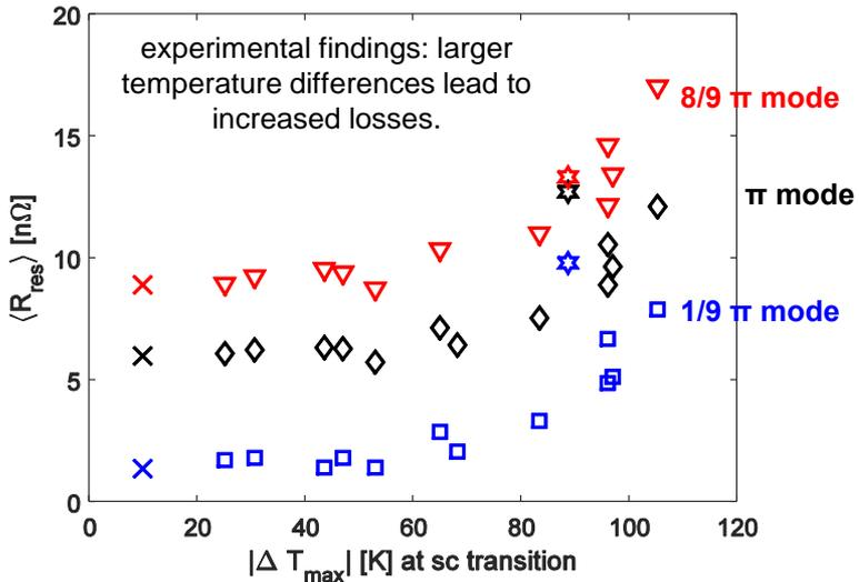
experimental evidence of correlation between additional losses in TESLA 9-cell cavities with high temperature gradients during cool-down
