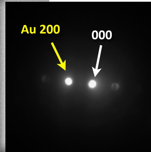
Electron diffraction image using conventional 200 keV TEM
