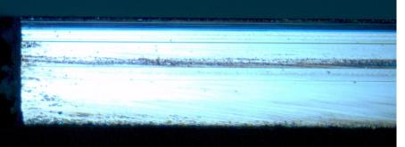
After cutting surface not suitable for edge TCT
