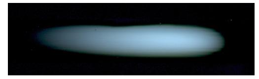
Polishing with paste: remove all scratches; final result is a smooth surface without scratches
