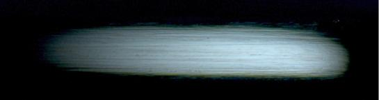
Polishing with lapping film: remove large scratches; the final result should be a homogeneous surface with only thin scratches
