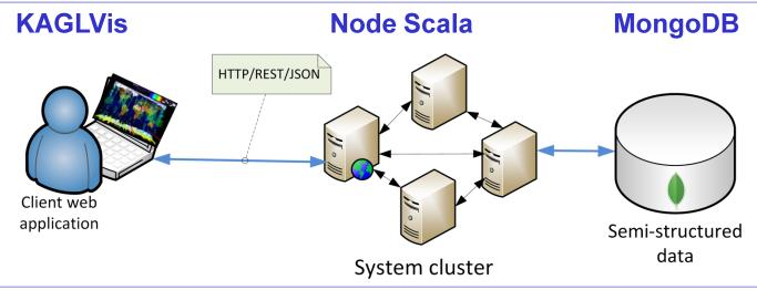
A horizontally-scalable multiprocessing platform based on Node.js
