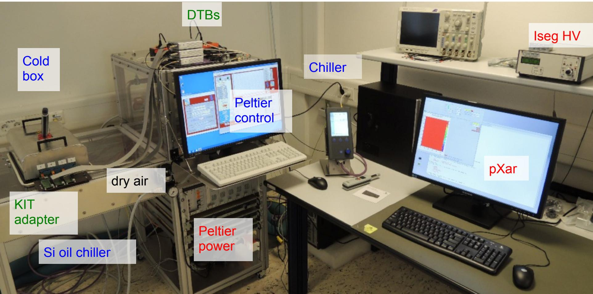
PC provides temperature control of the cold box and second computer is used for data taking
