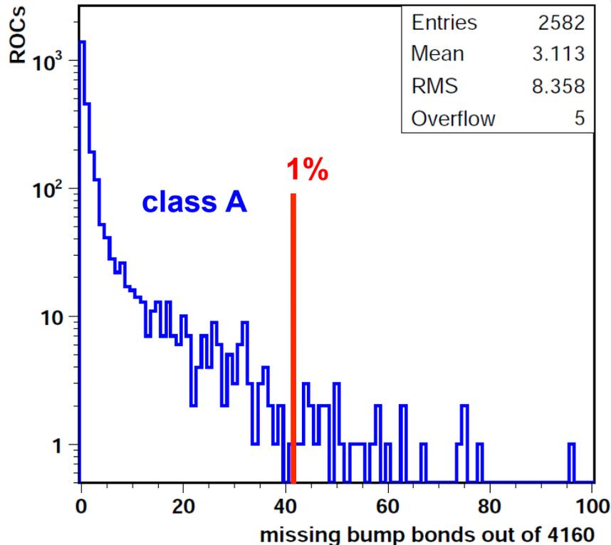
➤ Bump bond connection and response for each pixel is checked
