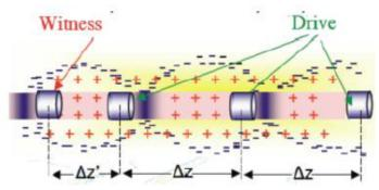
A train of three electron bunches (driver bunches) is sent through a capillary discharge
