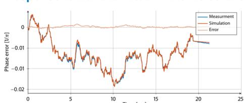
To acquire a mathematical model of the MLO control system it is excited with a PRBS signal and with band limited white noise. From the response the system above can be identified. This description can be used to calculate a controller using model based approaches. The signals in the model above are timing differences with respect to a perfect clock. Main control target is to minimize  $y$  while keeping  $u$  in an allowed range.
