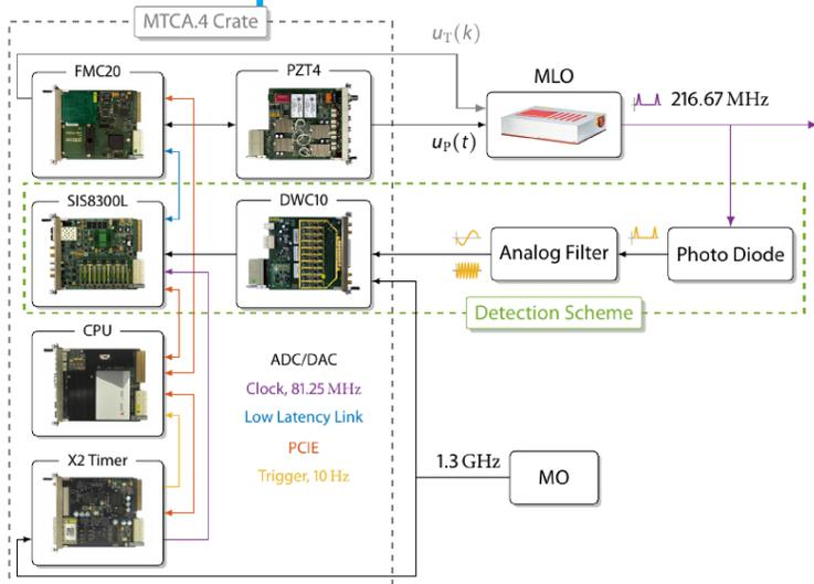
The MLO, a OneFive Origami laser, generates the 216.67 MHz laser pulse train. This optical signal is delivered to several end stations. Using a fast photo diode the optical pulses are converted and fed into the Phase Detection Scheme shown below. The SIS8300L AMC Board is used to sample the analog signals and run the control algorithm. A FMC20 AMC receives the controller output over a Low Latency Link and uses a PZT4 RTM to excite the piezo crystal inside the laser, tuning its repetition rate.
