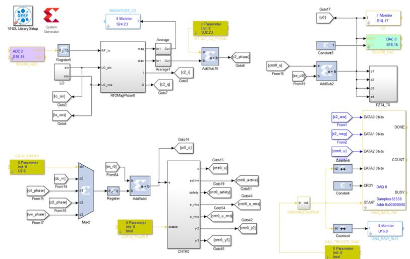
The application part of the firmware which includes e.g. the control algorithm is developed in MATLAB Simulink with Xilinx System Generator and the in house developed Rapid-X toolbox. Advantages of this scheme are:
