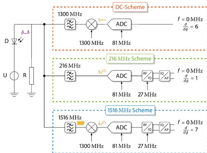
The controller minimizes the phase difference between MLO and MO. The DC-Scheme mixes the 6<sup>th</sup> harmonic of the pulse train with the MO frequency to generate a DC signal which gives the phase error. The 216MHz-Scheme directly samples the 216MHz fundamental of the pulse train and the 1516MHz-Scheme the 7<sup>th</sup> harmonic mixed with the MO signal. The phase is extracted by an IQ-Detection and Magnitude/Phase calculation.
