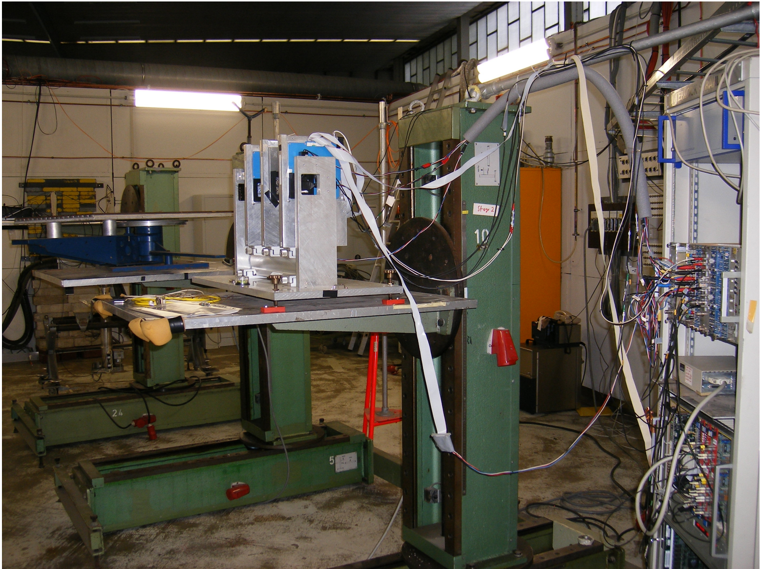
the ZEUS MVD telescope in test beam chamber 22
