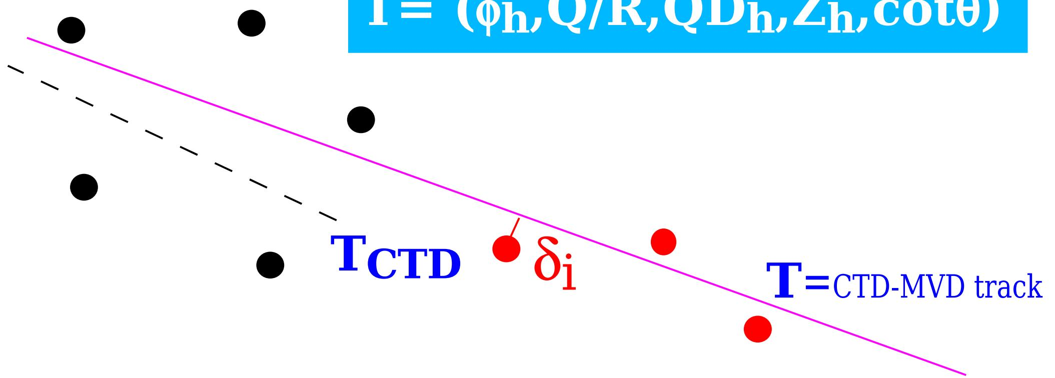
$$\chi^2 = (T_{ctd} - T)^t V_{ctd}^{-1} (T_{ctd} - T) + \sum \text{BMVD} \frac{\delta_i^2}{\sigma_i^2}$$
